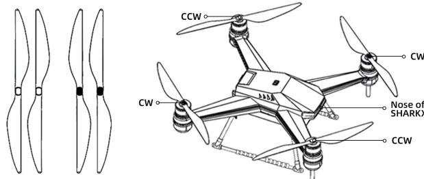
**CW Propeller Installation**
