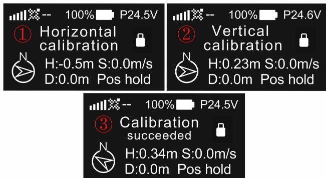
**Step 3:** When the screen shows “Vertical calibration”, hold the drone vertically with its nose downwards and start rotating. The RC will emit a short beep indicating the horizontal calibration has succeeded. Then the screen will show “Calibration succeeded”.
