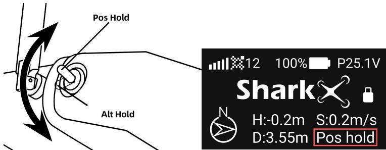
**Notice** when both joysticks are centered, if on **Pos Hold** mode, the drone will hover at the current position, and if on **Alt Hold** mode, the drone might get pushed away from the current position by wind.
