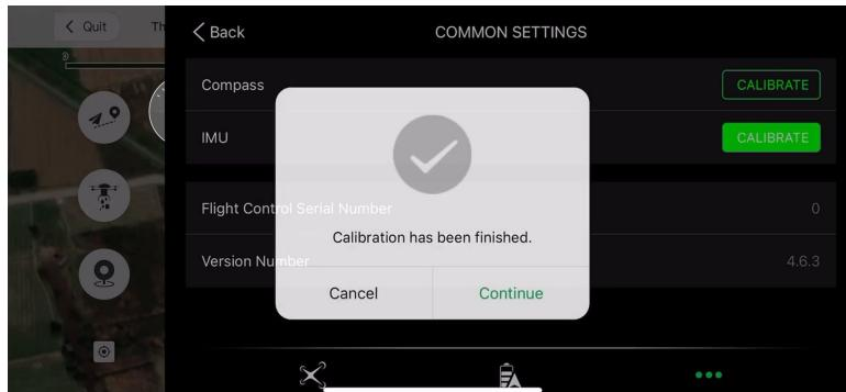
**Notice** if the SharkX appears to shift forward or backward, does uncontrolled circles or does not respond to controls, or flies erratically – land immediately and re-calibrate the compass. If problem still persists, this could be a number of factors including external magnetic or radio interference so contact local distributor/dealer and seek help.
