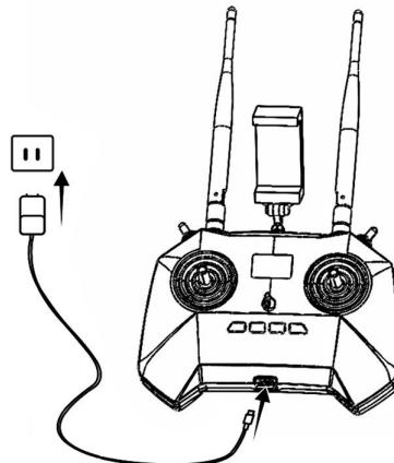
It takes approx. 3.5 hours to fully charge the controller. When it is fully charged:
