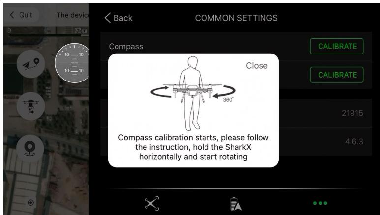
**Step 3:** Following the voice prompt, hold the drone horizontally with its nose outwards and complete the horizontal calibration. And then hold the drone vertically with its nose downwards and complete the compass calibration.
